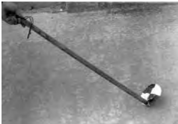
Figure 6. A Secchi disk is used to estimate the concentration of algae in water.
