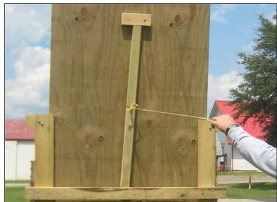
Figure 6. A hinge connects two pieces of wood, which rest on a block holding up the door. Just a light tug with a string causes the hinge to collapse and the door to fall. Photo by Becky McPeake, University of Arkansas.
